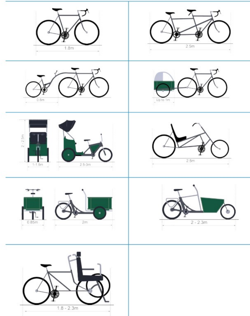
Figure 5.2: Typical dimensions of cycles
